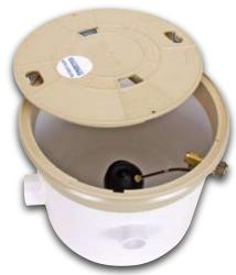
The Waterco Automatic Water Leveller is placed in the ground at a convenient location near the pool and plumbed to a separate pool inlet and also to the fresh water supply. The leveller remains inactive until the pool water level drops below or rises above the correct point at which time it will restore the right level by adding or draining water as the situation requires.
